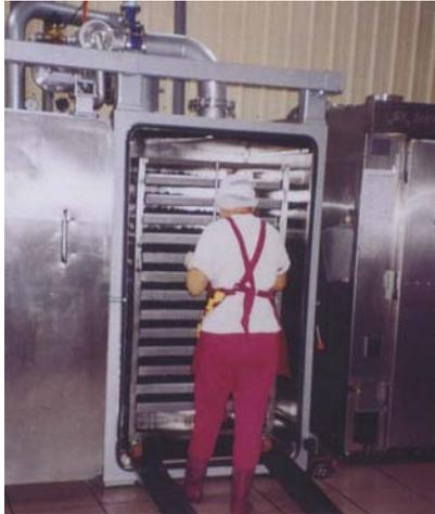
Example of 175 Kg trolley loading vacuum cooler being loaded
